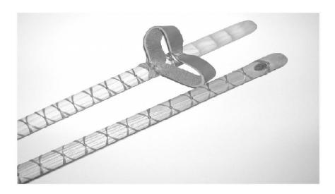
Trim the tied ends even and attach them to the shaft using a little glue or heat it with a match and melt it together.
